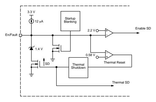
Figure 6. Enable/Fault Simplified Circuit
