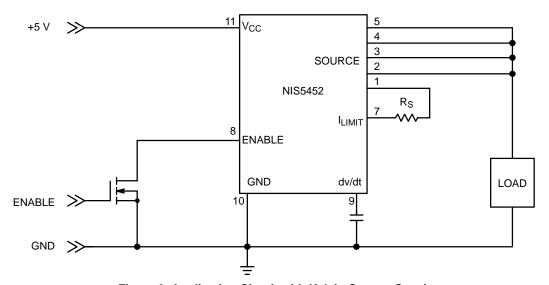
Figure 3. Application Circuit with Kelvin Current Sensing
