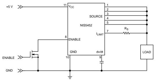
Figure 2. Application Circuit with Direct Current Sensing
