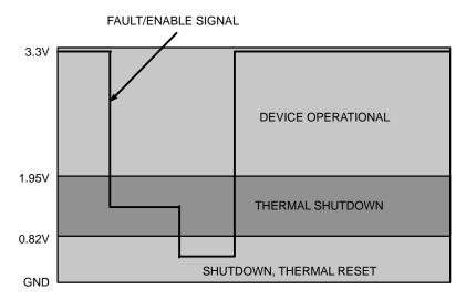
Figure 5. Enable/Fault Signal Levels
