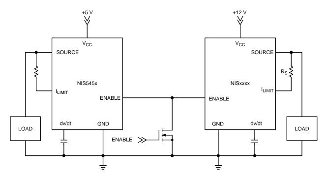
Figure 4. Common Thermal Shutdown
